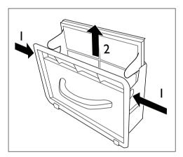
To clean the fluff filter: Remove filter from filter housing. To do this, press the pressure points on the sides and pull the filter frame up and out of the housing. Remove fluff from the fluff filter with a damp hand.
